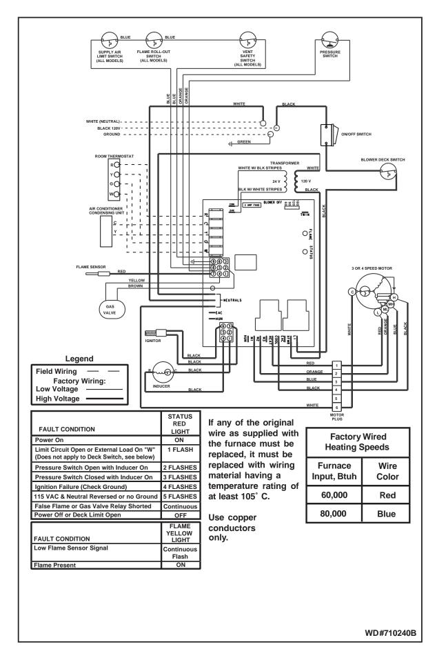
Figure 30. Downflow Furnace Wiring Diagram
